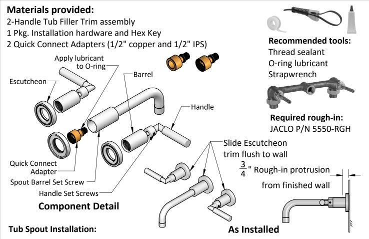
**Step 1:** Determine if the existing rough-in is either a 1/2" IPS or 1/2" copper sweat. The Spout rough-in pipe should protrude from the finished wall 3/4".
